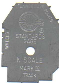
*NMRA mkIV standards gauge, checks loading gauge, platform height and RP25 rail and wheel standards.*
