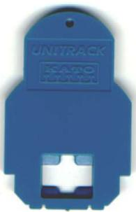
*Kato gauge for checking loading gauge, catenary height, platform height, also functions as 'Unijoiner' remover to remove joiners from Kato 'Unitrack'. Comes together with a rerailer ramp.*
